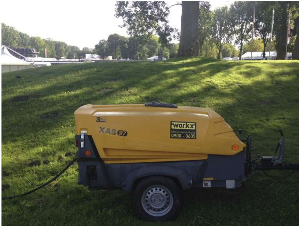
The compressor used to operate the bubble finish.
