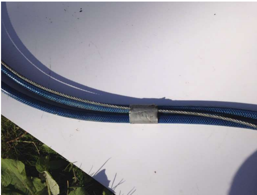
The two bubble finish hoses attached to the steel wire.
