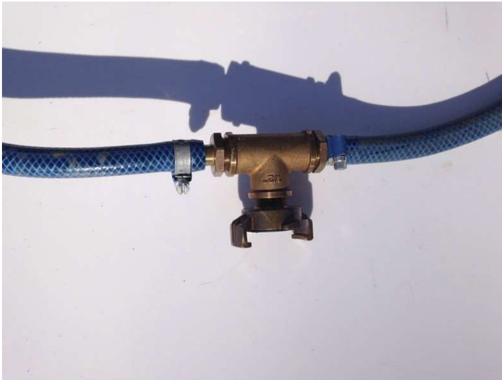
The connection point of the pressured air. Here the two sections of the bubble finish split out.
